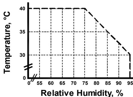
**Important:** For rated performance at 10 LPM do not operate the Oxygen concentrator above the indicated boundaries. Operating at flow rates less than 10 LPM will tolerate higher temperature/humidity conditions.
