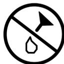
**"Use No Oil or Grease"** A spontaneous and violent ignition may occur if oil, grease or other petroleum substances come into contact with oxygen under pressure. Keep these substances away from the oxygen concentrator, tubing and connections and any other oxygen source. **Do Not** use any petroleum based or other lubricants unless recommended by SeQual Technologies Inc.
